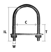
IL = Inside Length T = Thread Length W = Thread SizeC = Width Between Legs
